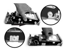
6. (1)Slide the hard drive into the front Base Plate first and (2) press down on the hard drive, make sure all 4 Anti-Shock Mounts sit inside the Support Slot.
